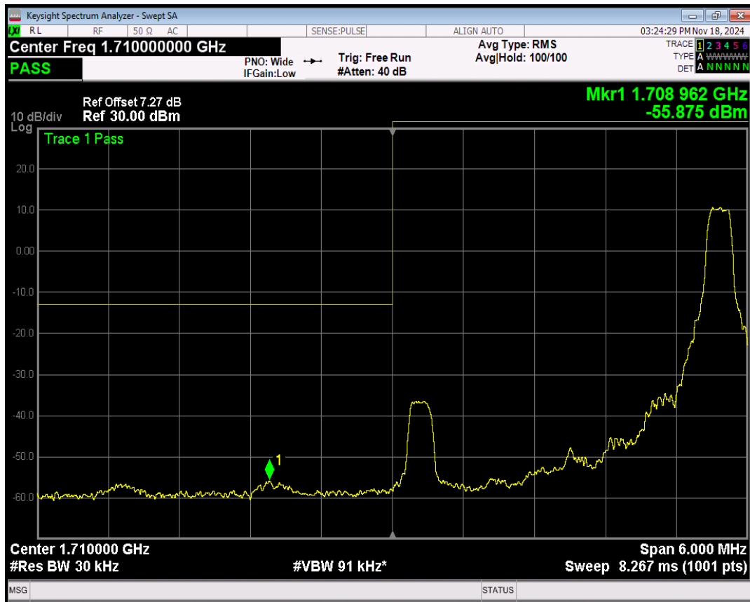
Band66 QPSK BW=3MHz Channel=131987 RB Size=15 Position=#0
