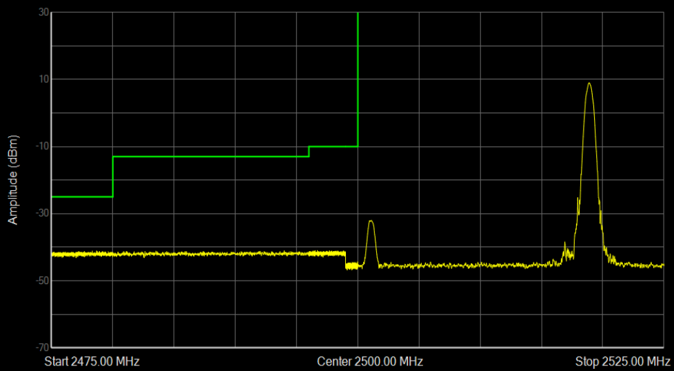
Band7 16QAM BW=20MHz Channel=20850 RB Size=1 Position=#Max
