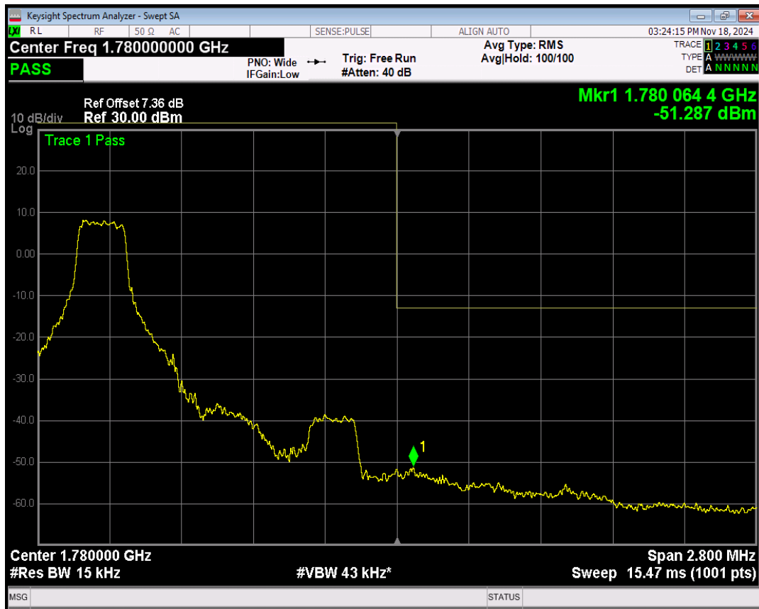
Band66 16QAM BW=1.4MHz Channel=132665 RB Size=1 Position=#Max
