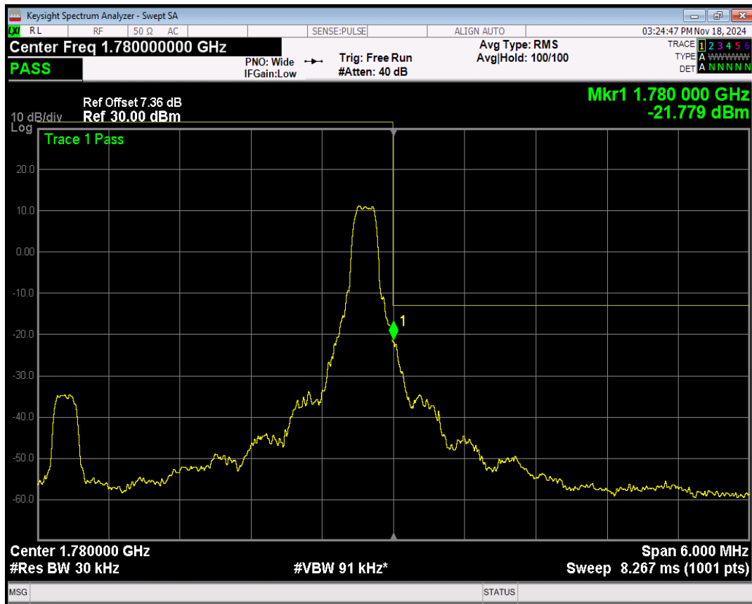
Band66 QPSK BW=3MHz Channel=132657 RB Size=15 Position=#0
