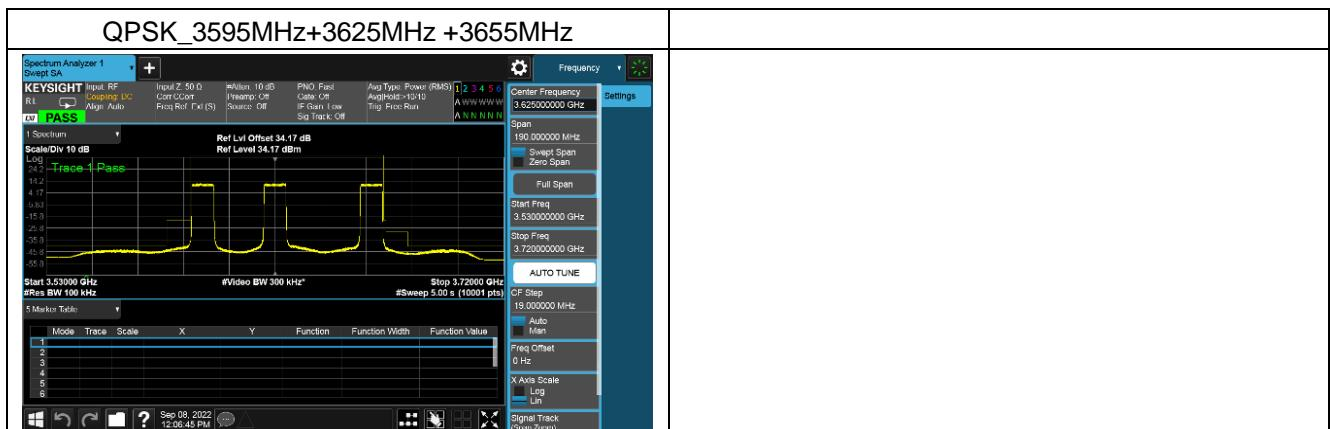
1. Remark: For 4\*4MIMO, one of ANT ports was measured and the limit shall be reduced by  $10\lg(4)$ , so the limit was calculated to  $-19\text{dBm}/\text{MHz}$  within 0-10 megahertz above/below the upper/lower SAS-assigned channel edge and  $-31\text{ dBm}/\text{MHz}$  at all frequencies greater/less than 10 megahertz above/below the upper/lower SAS assigned channel edge in order to determine the test result conveniently.
