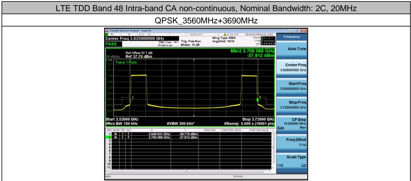
1. Remark: For 4\*4MIMO, one of ANT ports was measured and the limit shall be reduced by  $10\lg(4)$ , so the limit was calculated to -19dBm/MHz within 0-10 megahertz above/below the upper/lower SAS-assigned channel edge and -31 dBm/MHz at all frequencies greater/less than 10 megahertz above/below the upper/lower SAS assigned channel edge in order to determine the test result conveniently.
