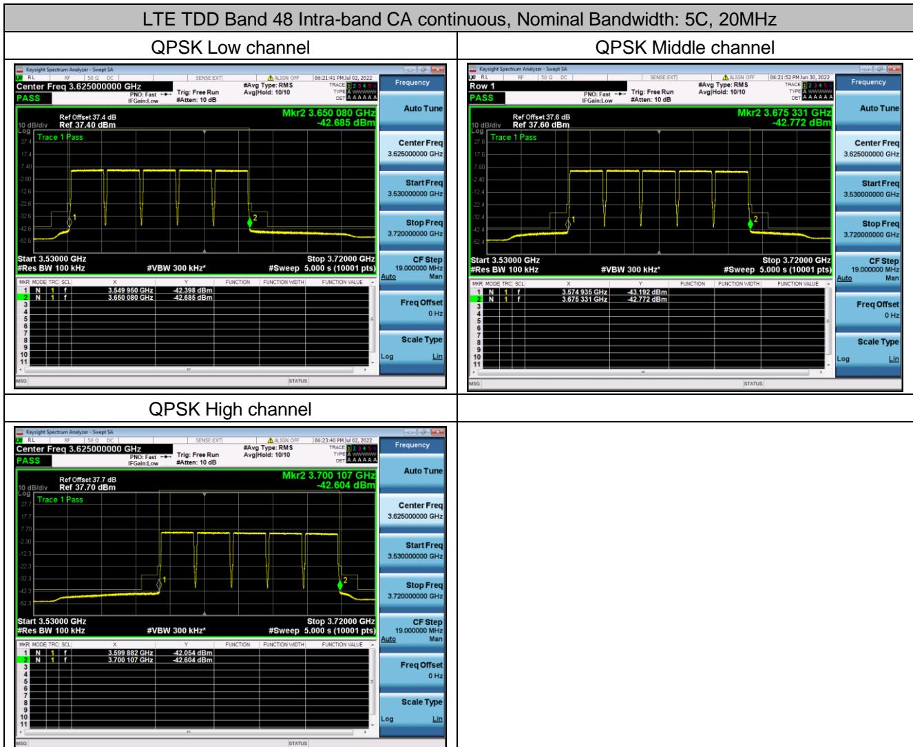
1. Remark: For 4\*4MIMO, one of ANT ports was measured and the limit shall be reduced by  $10\lg(4)$ , so the limit was calculated to -19dBm/MHz within 0-10 megahertz above/below the upper/lower SAS-assigned channel edge and -31 dBm/MHz at all frequencies greater/less than 10 megahertz above/below the upper/lower SAS assigned channel edge in order to determine the test result conveniently.
