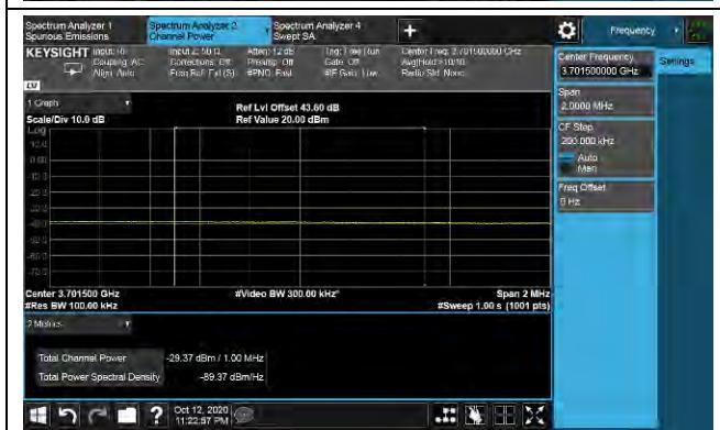
LTE TDD Band 48, Nominal Bandwidth: 20MHz \_16QAM Low channel
