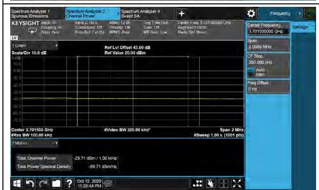
LTE TDD Band 48, Nominal Bandwidth: 20MHz \_256QAM Low channel
