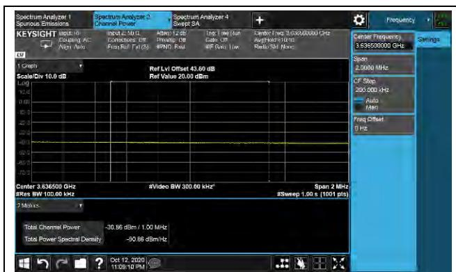
LTE TDD Band 48, Nominal Bandwidth: 20MHz\_QPSK High channel
