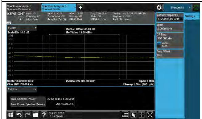
LTE TDD Band 48, Nominal Bandwidth: 5MHz \_256QAM High channel
