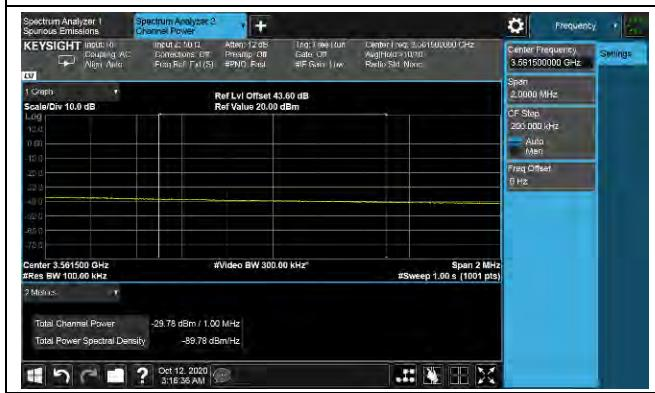
LTE TDD Band 48, Nominal Bandwidth: 10MHz \_QPSK Middle channel
