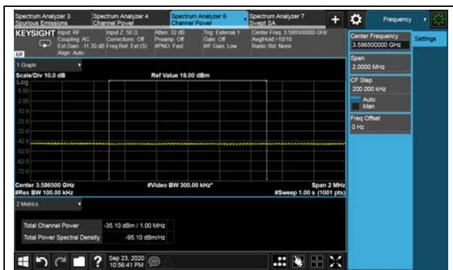
LTE TDD Band 48 Intra-band CA continuous, Nominal Bandwidth: 15M+20M QPSK Middle channel
