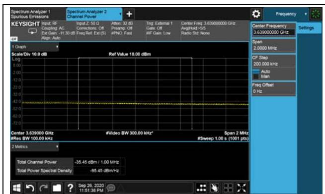
LTE TDD Band 48 Intra-band CA non-continuous, Nominal Bandwidth: 5M+15M+20M QPSK High channel
