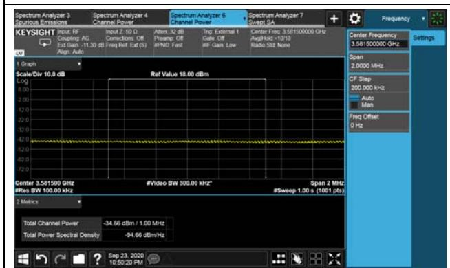
LTE TDD Band 48 Intra-band CA continuous, Nominal Bandwidth: 10M+20M QPSK Middle channel
