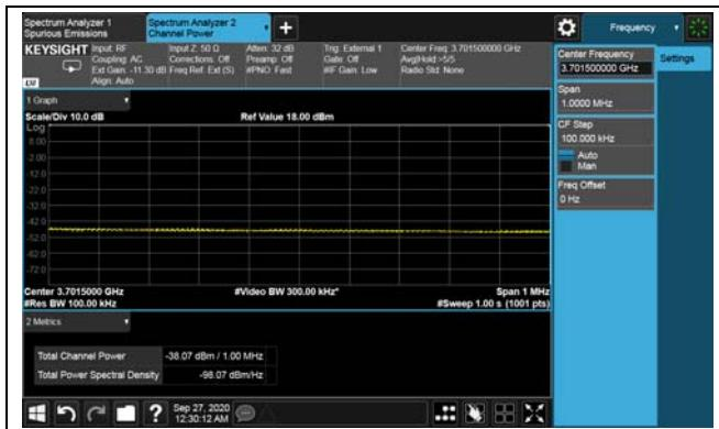
LTE TDD Band 48 Intra-band CA non-continuous, Nominal Bandwidth: 5M+10M+20M QPSK Low channel
