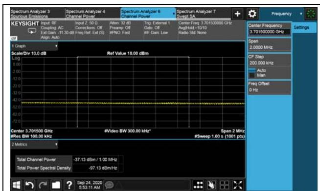
LTE TDD Band 48 Intra-band CA continuous, Nominal Bandwidth: 10M+20M QPSK Low channel
