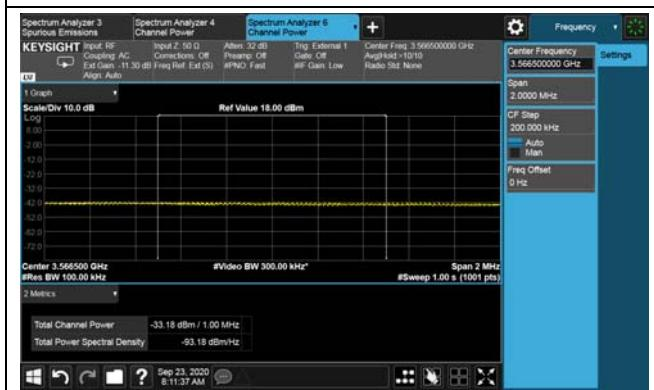
LTE TDD Band 48, Nominal Bandwidth: 15MHz Single carrier\_QPSK Middle channel
