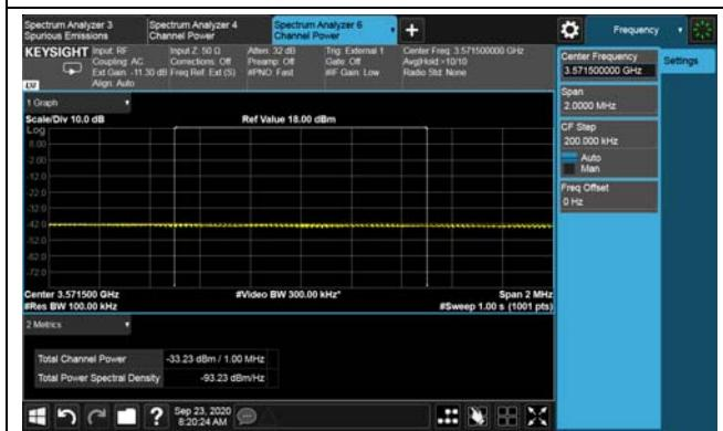
LTE TDD Band 48, Nominal Bandwidth: 20MHz\_Single carrier\_64QAM Middle channel
