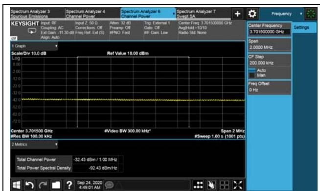
LTE TDD Band 48, Nominal Bandwidth: 15MHz\_Single carrier\_QPSK Low channel
