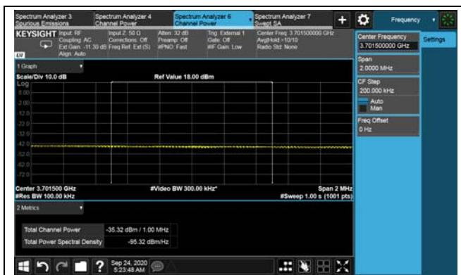
LTE TDD Band 48, Nominal Bandwidth: 20MHz\_Single carrier\_64QAM Low channel
