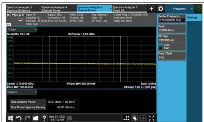
LTE TDD Band 48, Nominal Bandwidth: 10MHz\_Single carrier\_64QAM Low channel
