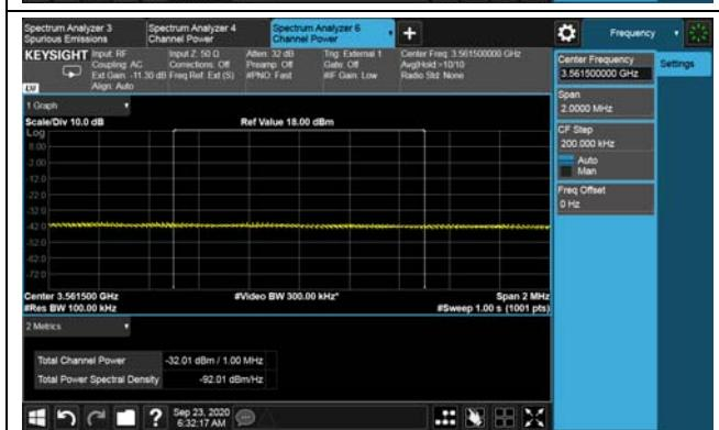
LTE TDD Band 48, Nominal Bandwidth: 10MHz Single carrier 64QAM Middle channel
