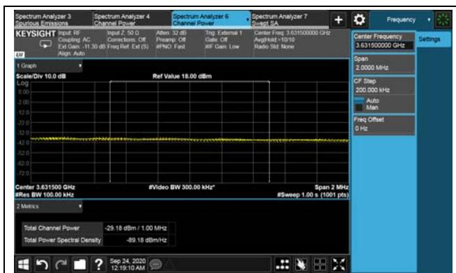
LTE TDD Band 48, Nominal Bandwidth: 10MHz\_Single carrier\_64QAM High channel
