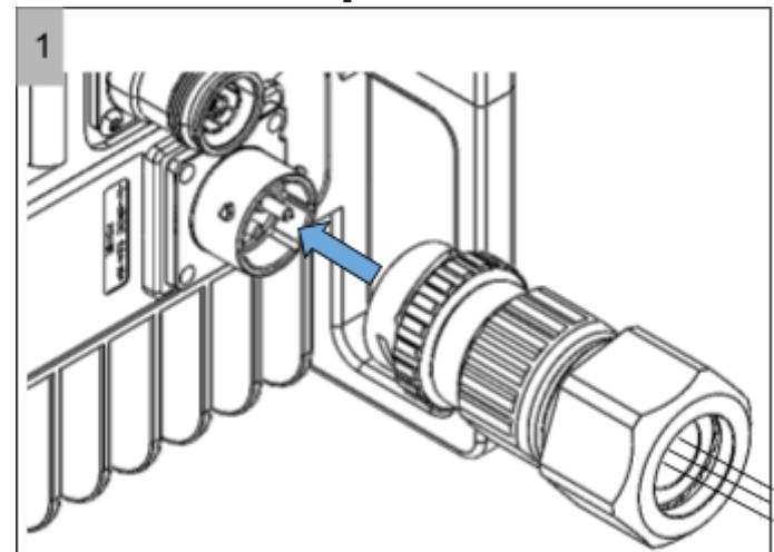
Note: Make sure that the keys on the cable match the grooves on the contact. (Fit A to A, B to B and C to C.)
