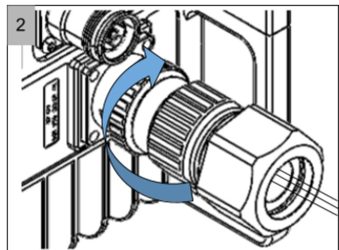
Note: Make sure that the connector is properly locked, to avoid bad connection and possible impact from rain or humidity.
