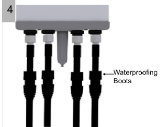
Note:Insert the rubber for waterproofing boot to the RF antenna ports.
