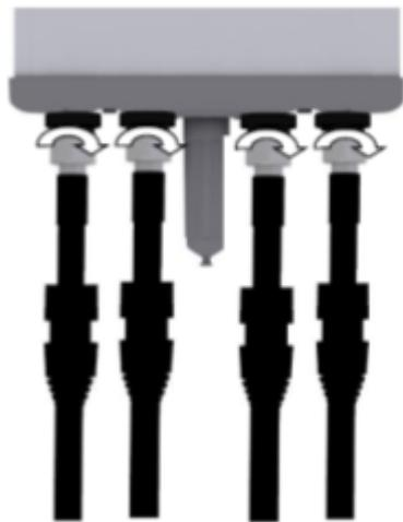
Note:Connect the cables to the RF antenna ports
