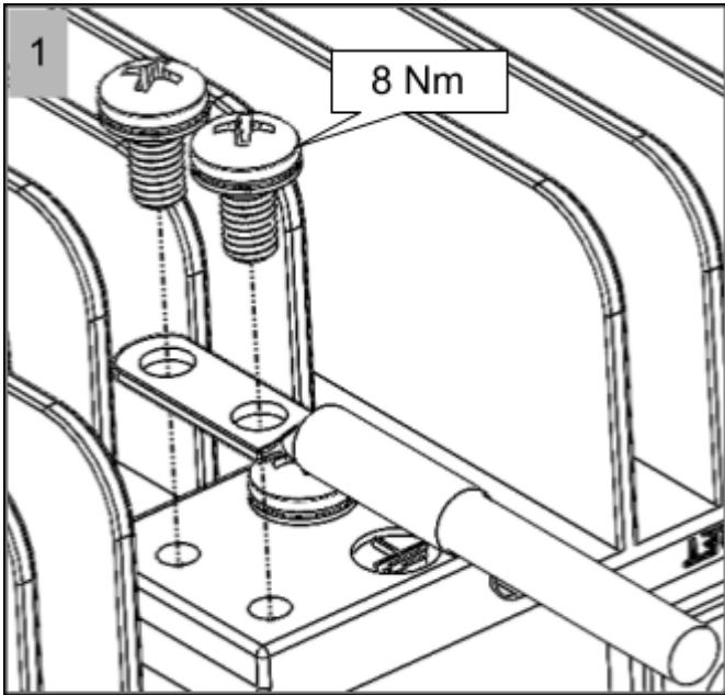
Note: The grounding cable size should be greater than 25 square millimeters and the terminal should satisfy 96h neutral salt fog test.
