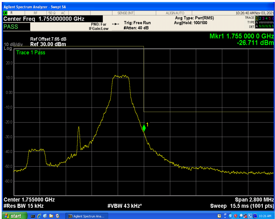
Band4 QPSK BW=3MHz Channel=19965 RB Size=1 Position=#0
