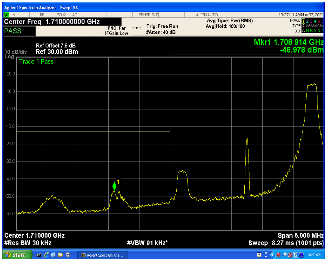
Band4 QAM16 BW=3MHz Channel=19965 RB Size=15 Position=#0
