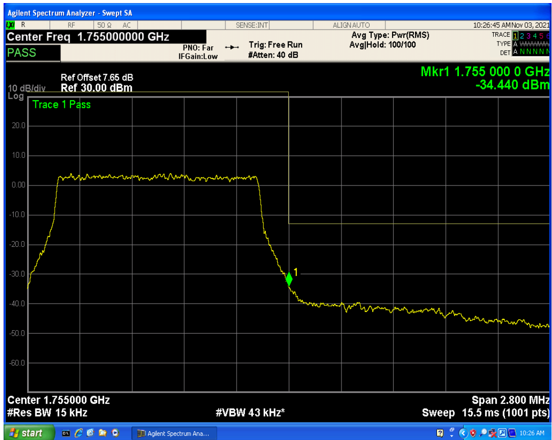
Band4 QAM16 BW=1.4MHz Channel=20393 RB Size=1 Position=#Max
