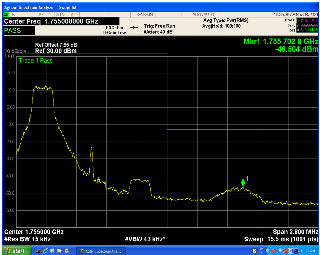
Band4 QPSK BW=1.4MHz Channel=20393 RB Size=6 Position=#0
