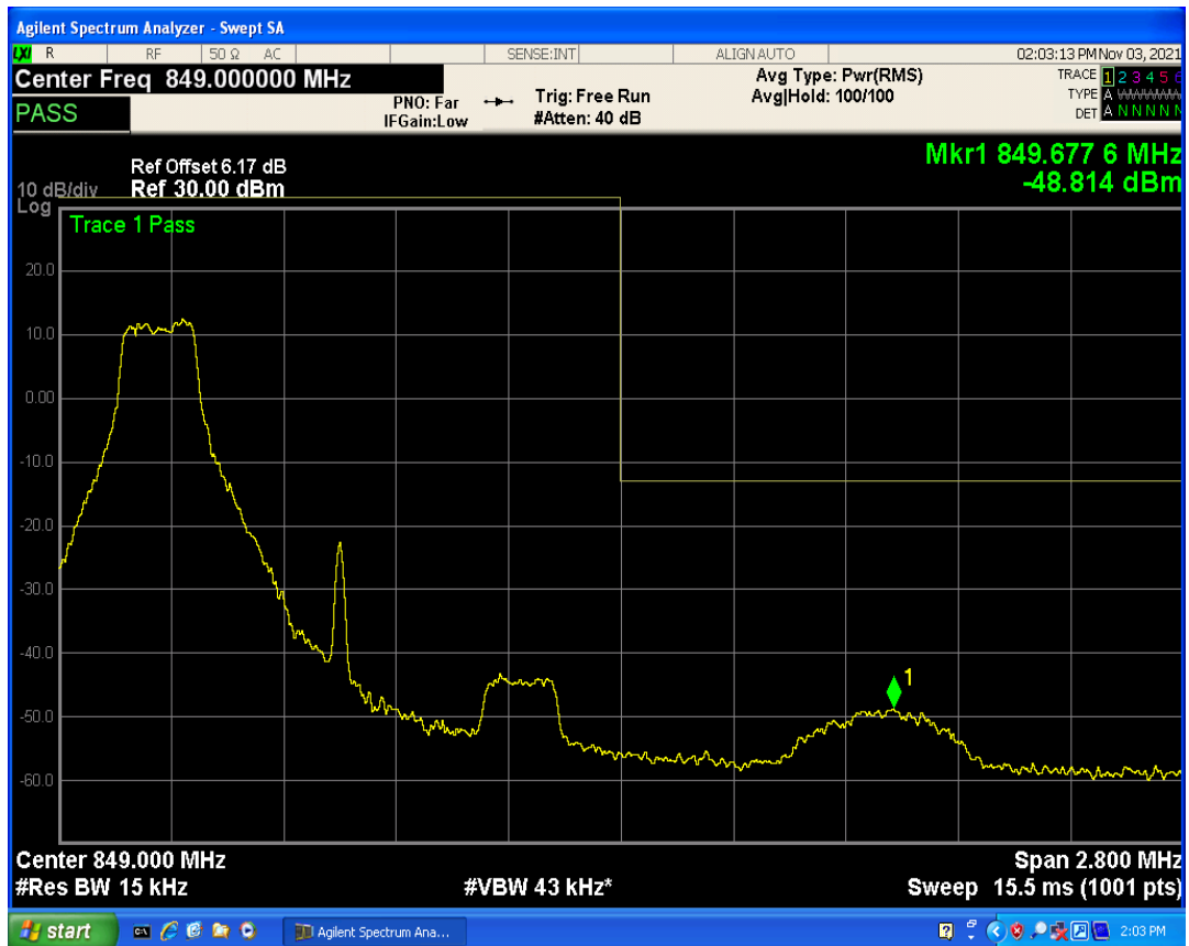
Band5 QPSK BW=1.4MHz Channel=20643 RB Size=6 Position=#0
