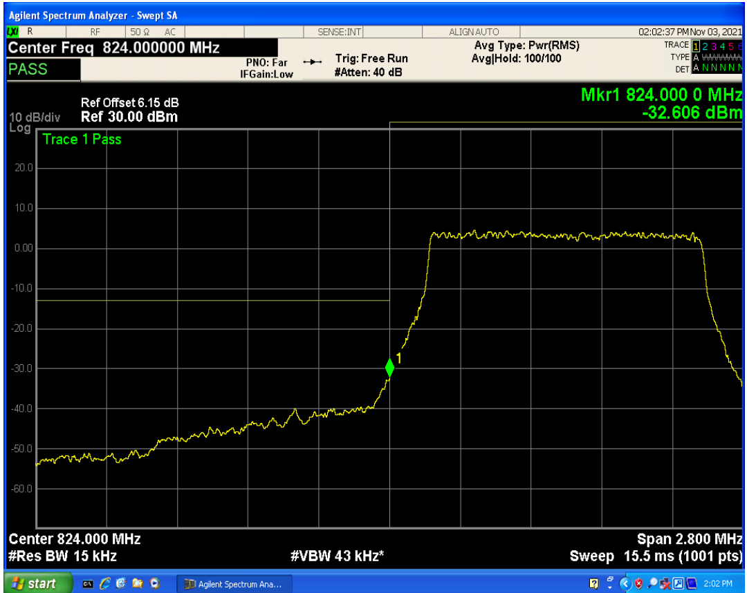
Band5 QAM16 BW=1.4MHz Channel=20407 RB Size=1 Position=#0
