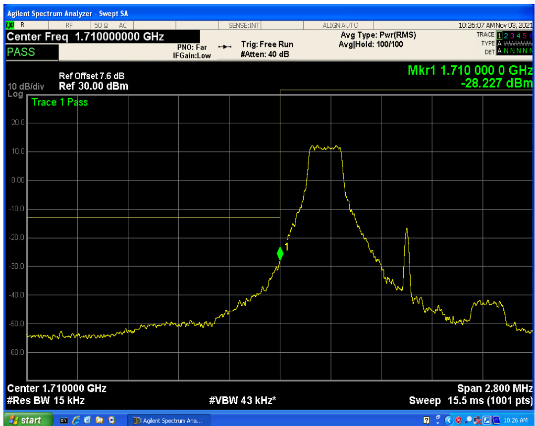
Band4 QPSK BW=1.4MHz Channel=19957 RB Size=6 Position=#0
