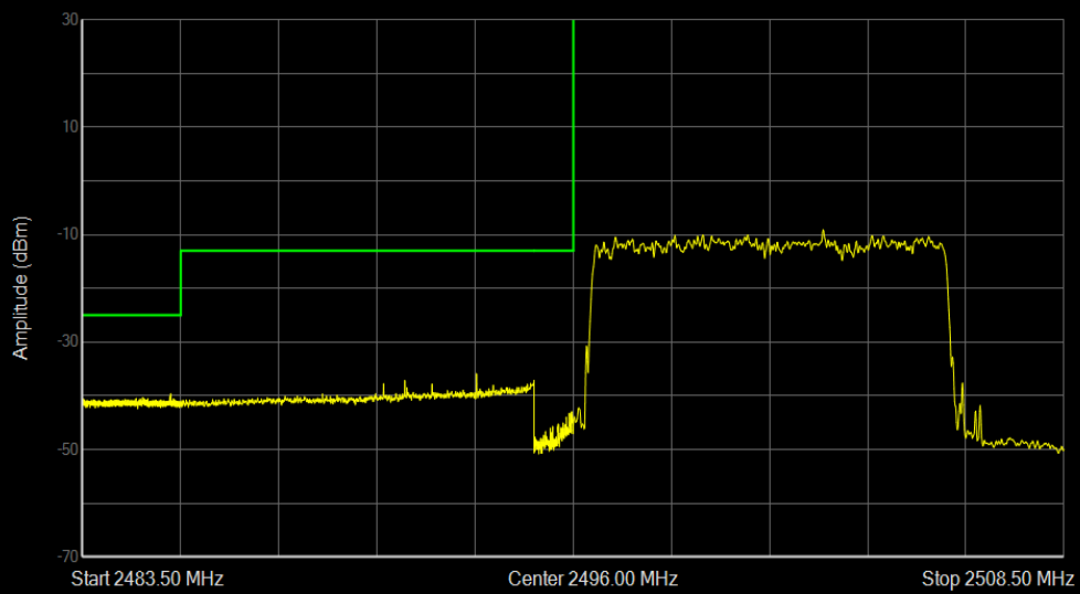
Band41 QPSK BW=10MHz Channel=39700 RB Size=50 Position=#0
