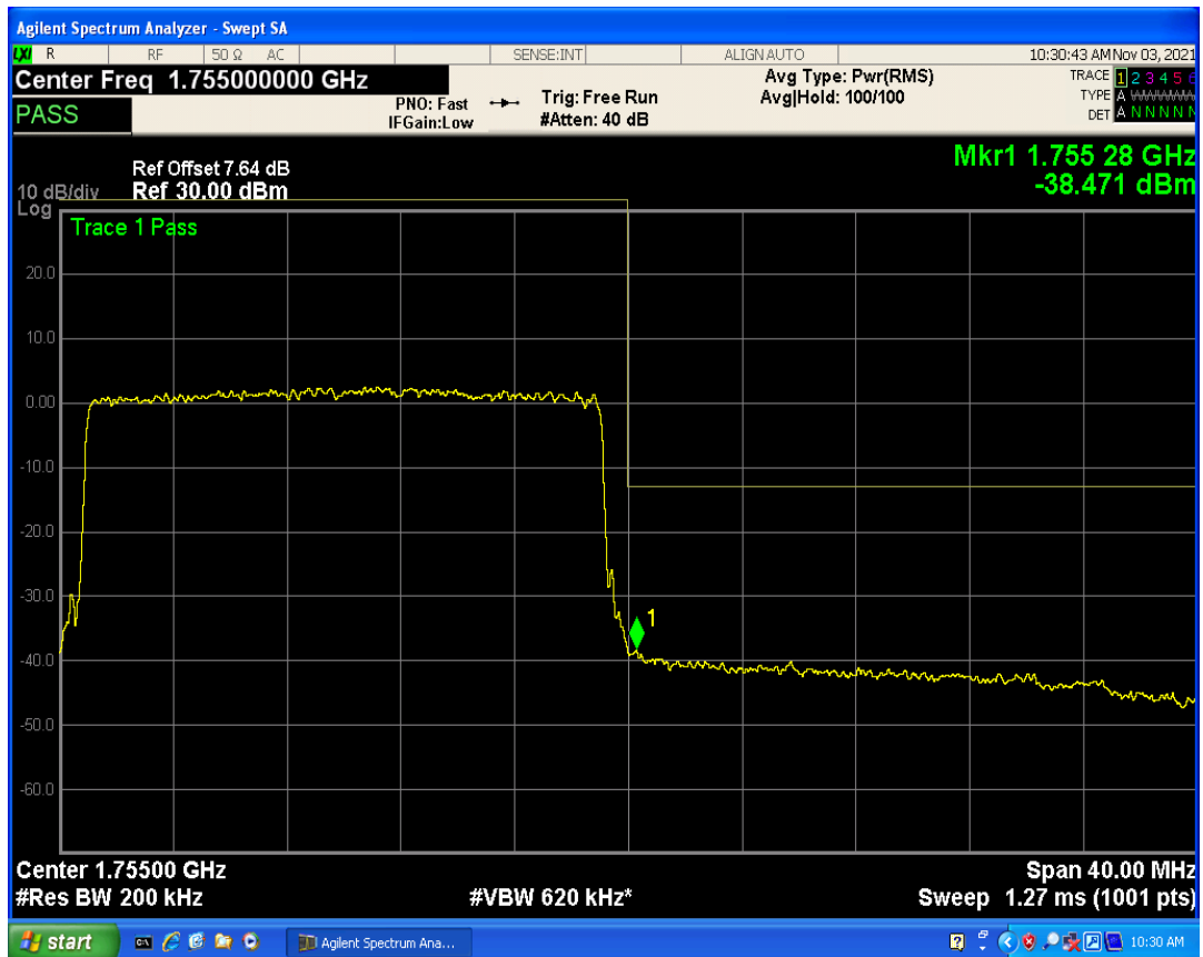
Band4 QAM16 BW=20MHz Channel=20300 RB Size=1 Position=#Max
