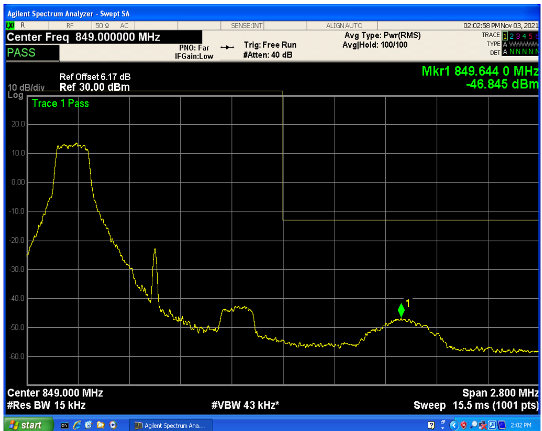
Band5 QAM16 BW=1.4MHz Channel=20407 RB Size=6 Position=#0
