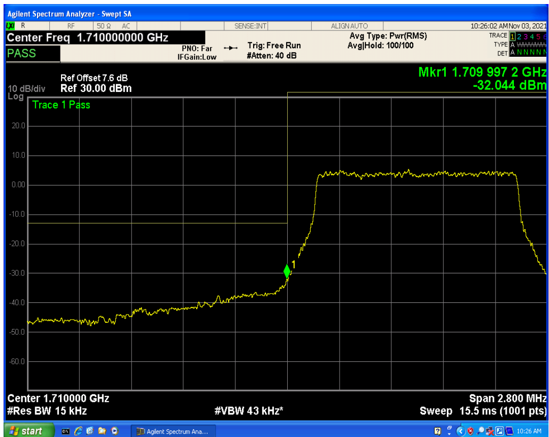
Band4 QAM16 BW=1.4MHz Channel=19957 RB Size=1 Position=#Max
