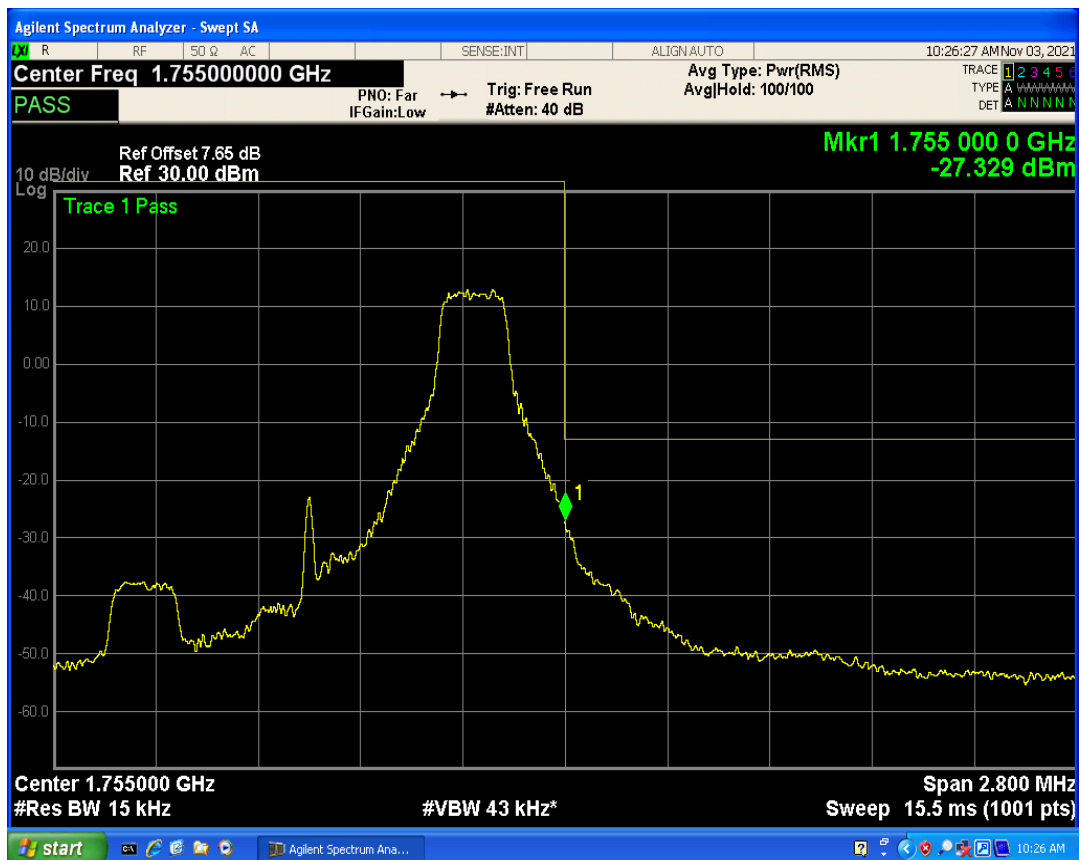
Band4 QAM16 BW=1.4MHz Channel=20393 RB Size=1 Position=#0
