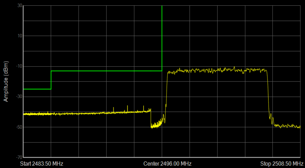
Band41 QAM16 BW=10MHz Channel=39700 RB Size=50 Position=#0
