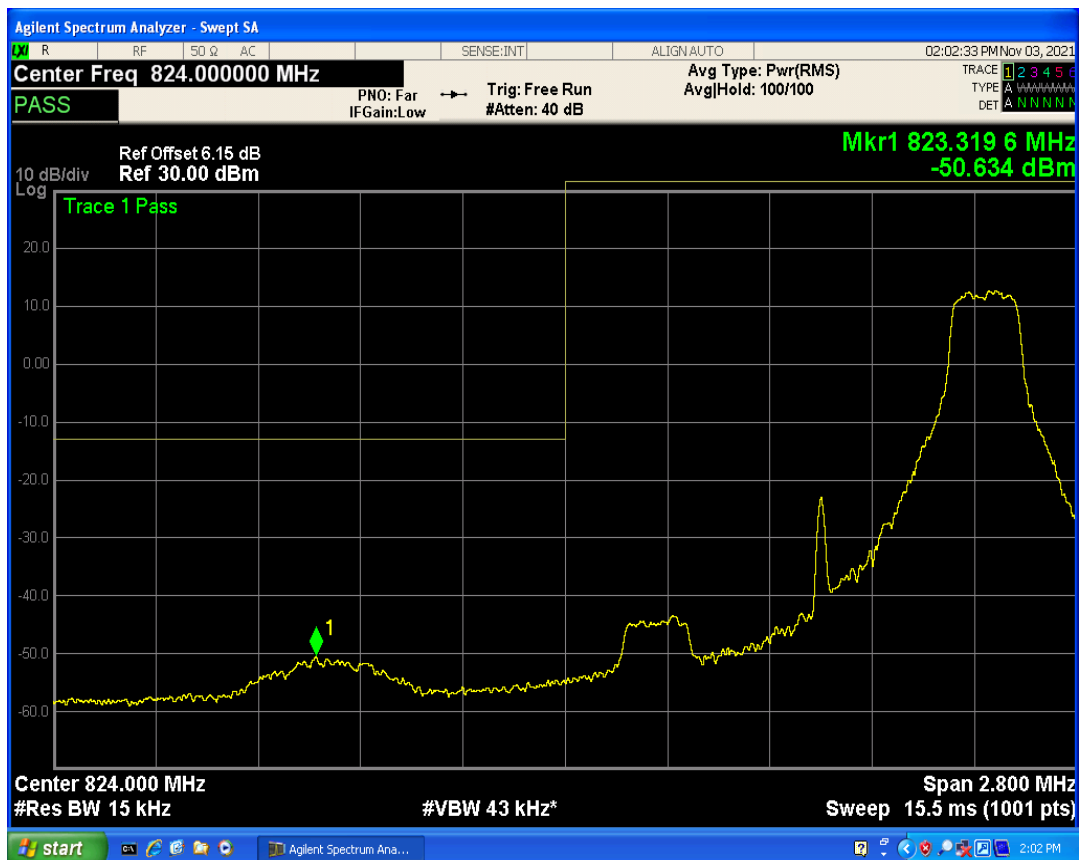
Band5 QPSK BW=1.4MHz Channel=20407 RB Size=6 Position=#0
