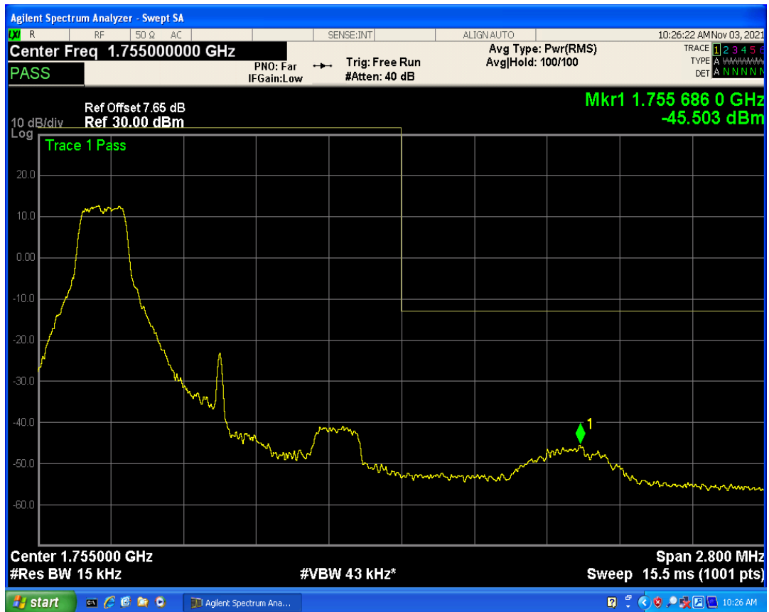
Band4 QPSK BW=1.4MHz Channel=20393 RB Size=1 Position=#Max
