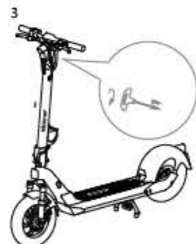
3. Use the hexagon wrench in the box to tighten the screws on both sides and the back of the handlebars.
