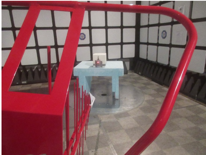
Photo 12: – Test Setup – 30MHz to 1GHz – Vertical Polarization (Radio Remote Control)
