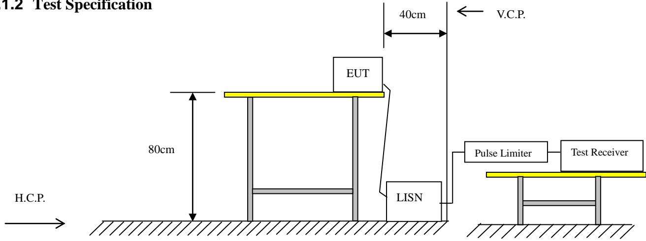
EUT was placed upon a wooden test table 0.8m above the horizontal metal reference plane and 0.4m from the vertical ground plane, and it was connected to an AMN. The closest distance between the boundary of the EUT and the surface of the AMN is 0.8m. All peripherals were connected to another AMN, and placed at a distance of 10cm from each other. A spectrum and receiver was connected to the RF output port of the AMN. Both average and quasi-peak value were detected.
