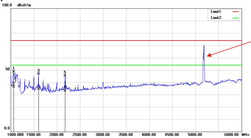
Fundamental Test with Band Rejection Filter
