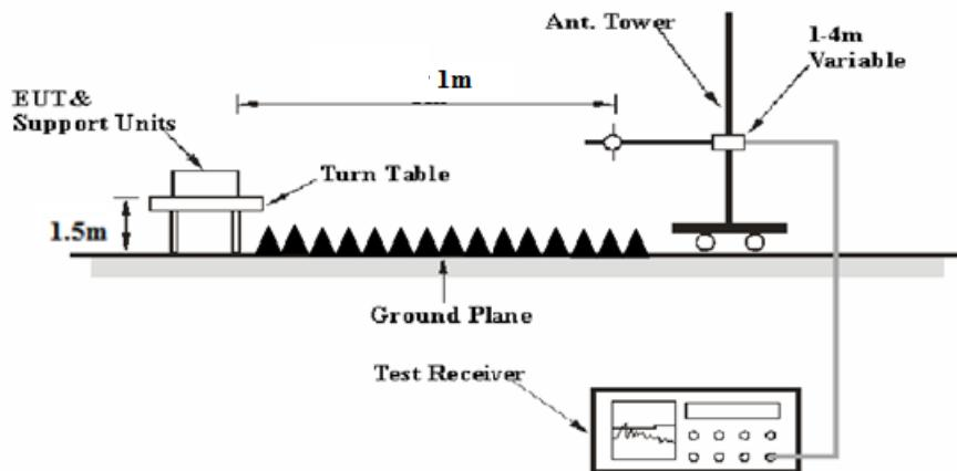
The radiated emission Below 1GHz tests were performed in the 10 meters chamber, above 1GHz tests were performed in the 3 meters chamber test site B, using the setup accordance with the ANSI C63.10-2013. The specification used was the FCC 15.209, and FCC 15.407 limits.
