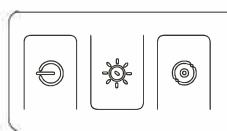
1. Short press (&lt;1s) on/off key, switch the switch mode, short press once to turn on the light strip, press again to turn off. In the non-reset state, it will memorize the state of the light strip before it was turned off last time.
