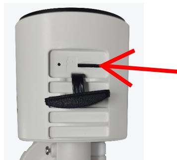
Remove plastic cover to open microSD card slot. Slide microSD Card into SD card slot.
