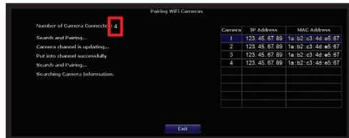
**NOTE:** You cannot exceed the number of Wireless NVR channels you have. If you have a 4 channel system, the maximum number of cameras you can have paired is 4.
