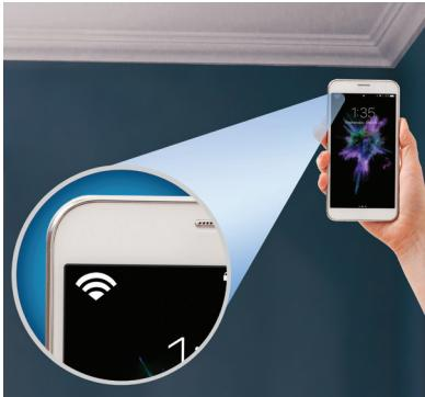
**NOTE:** Night Owl recommends using your cell phone to test the location for your Wi-Fi signal strength before installing the camera.
