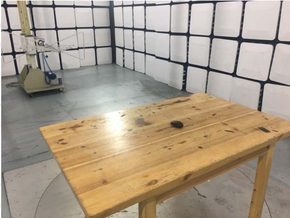
Photo of Radiation Emission Test
