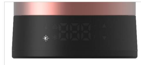
Short press the brightness button to change the brightness of the display.
