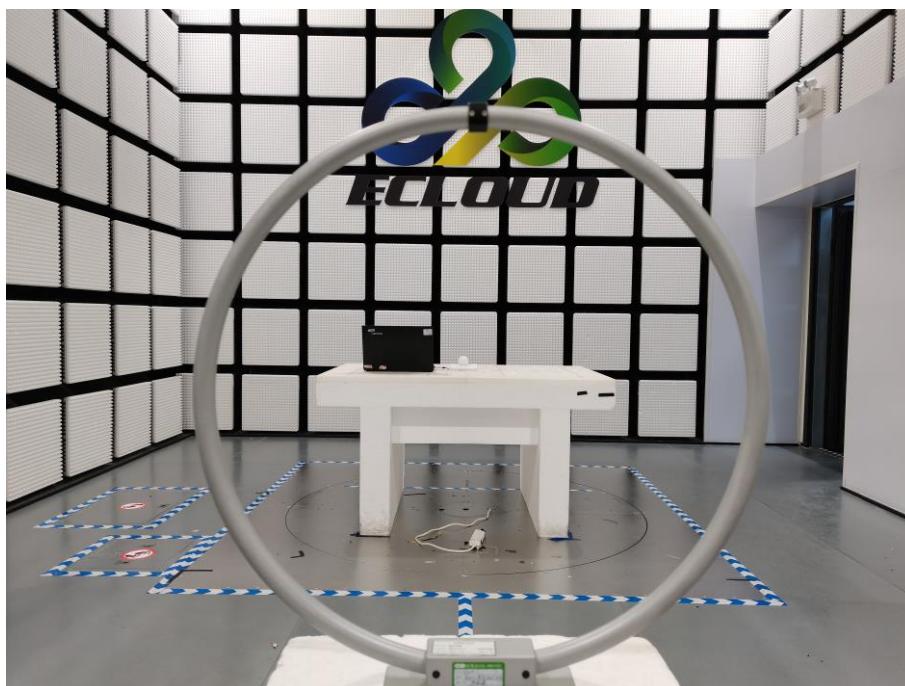
Fig. 1 Radiated emission setup photo(Below 30MHz)
