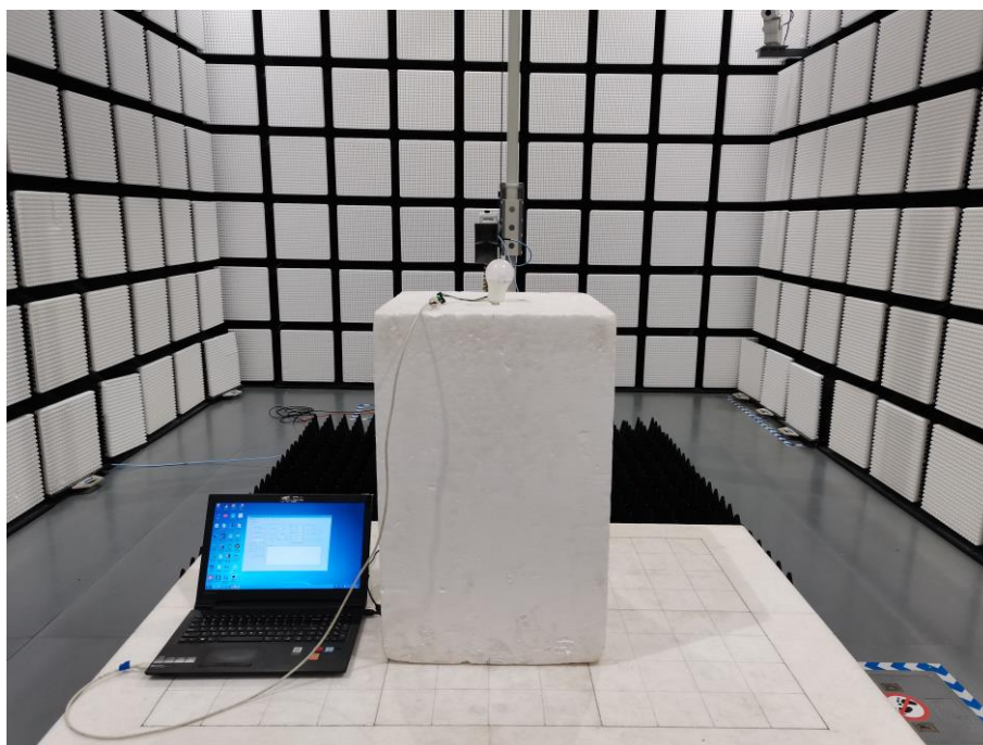
Fig. 3 Radiated emission setup photo(Above 1GHz)
