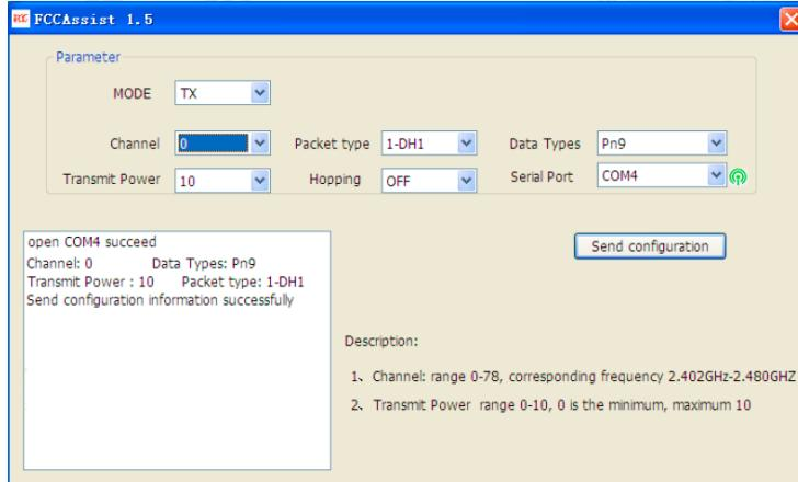
The test software was used to control EUT work in continuous TX mode, and select test channel, Wireless mode as below table
