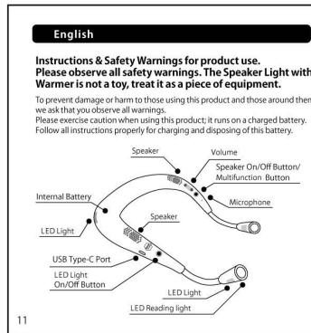
Input Power : DC 5V 1.0A (USB charging system)
