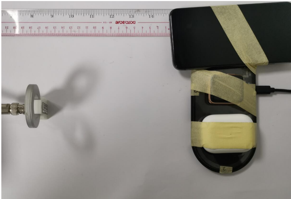
H-field Test Setup Photo of Position B(15cm)
