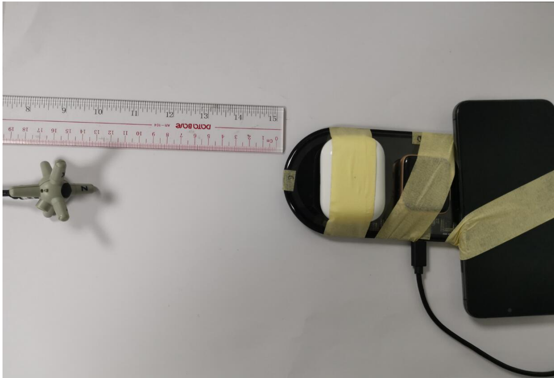
E-field Test Setup Photo of Position C(15cm)
