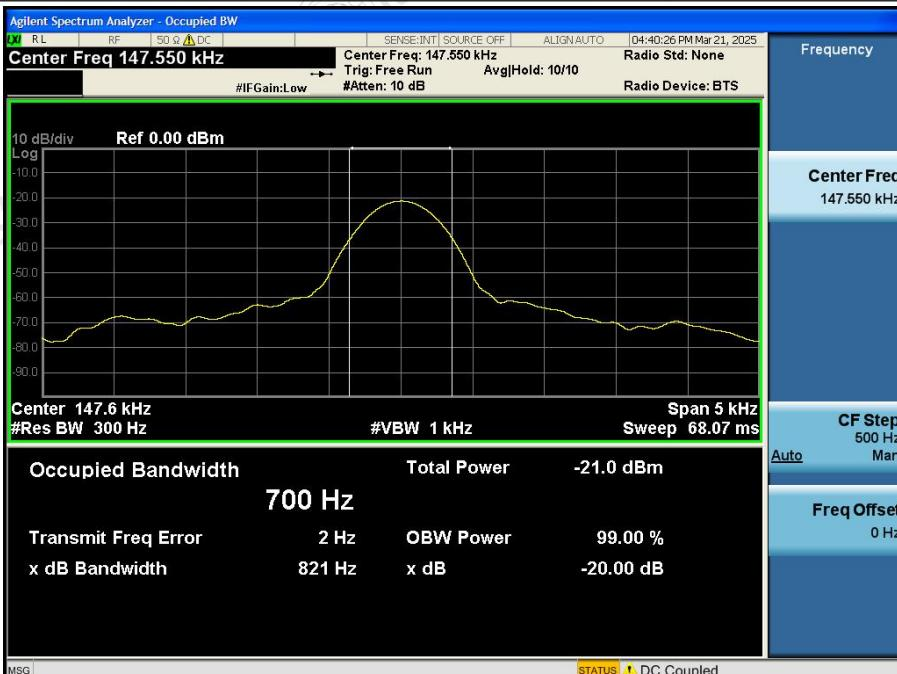
The screenshot shows the Agilent Spectrum Analyzer interface for an occupied bandwidth test. The center frequency is set to 147.550 kHz. The spectrum displays a single peak at 147.550 kHz. The occupied bandwidth is measured as 700 Hz. The 99% occupied bandwidth is measured as 821 Hz. The plot shows a reference level of 0.00 dBm and a span of 5 kHz. The measurement parameters are listed as follows:
