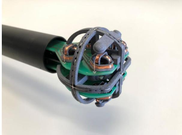
Test probe, without the casing
