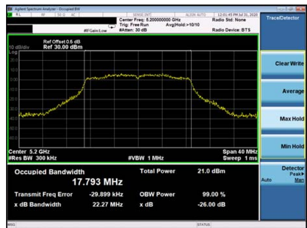
(802.11 n20) -26dB&99%Bandwidth plot on channel 40
