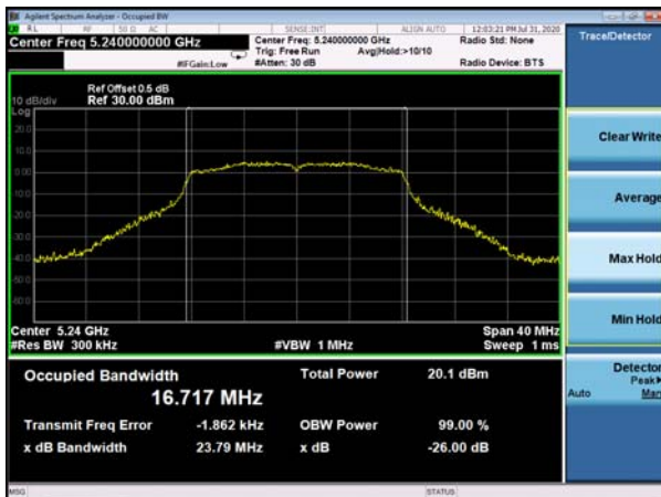
(802.11a) -26dB&99%Bandwidth plot on channel 48
