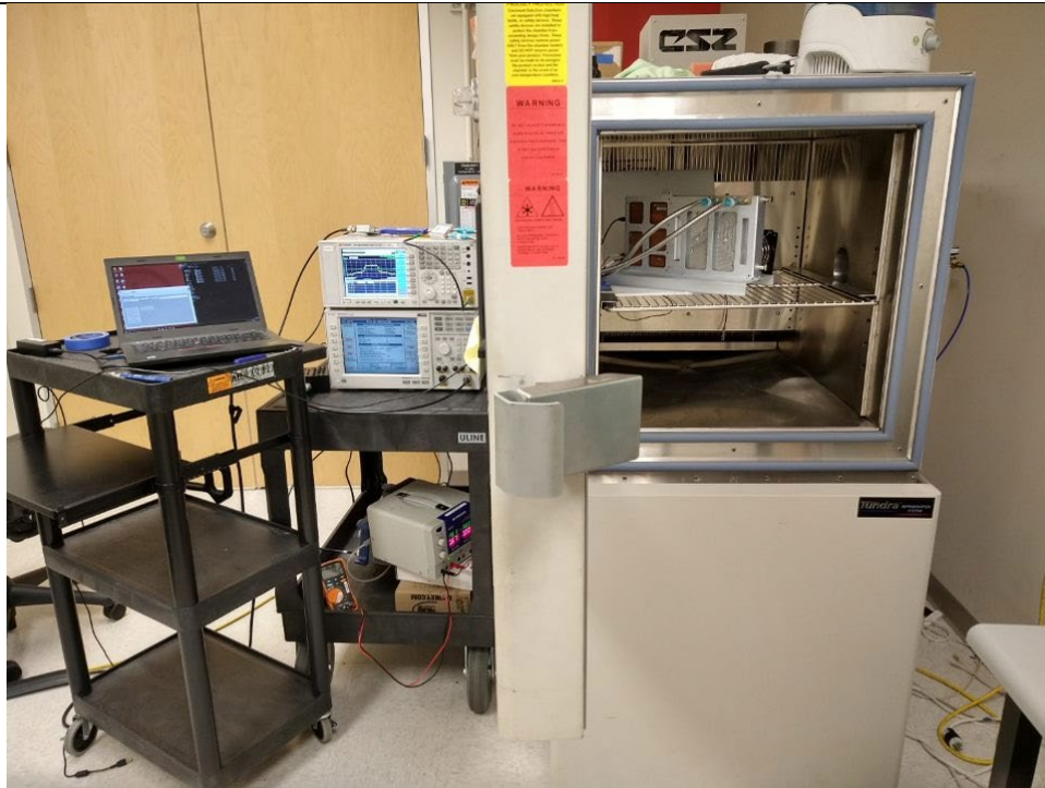
ANTENNA PORT CONDUCTED RF MEASUREMENT SETUP
