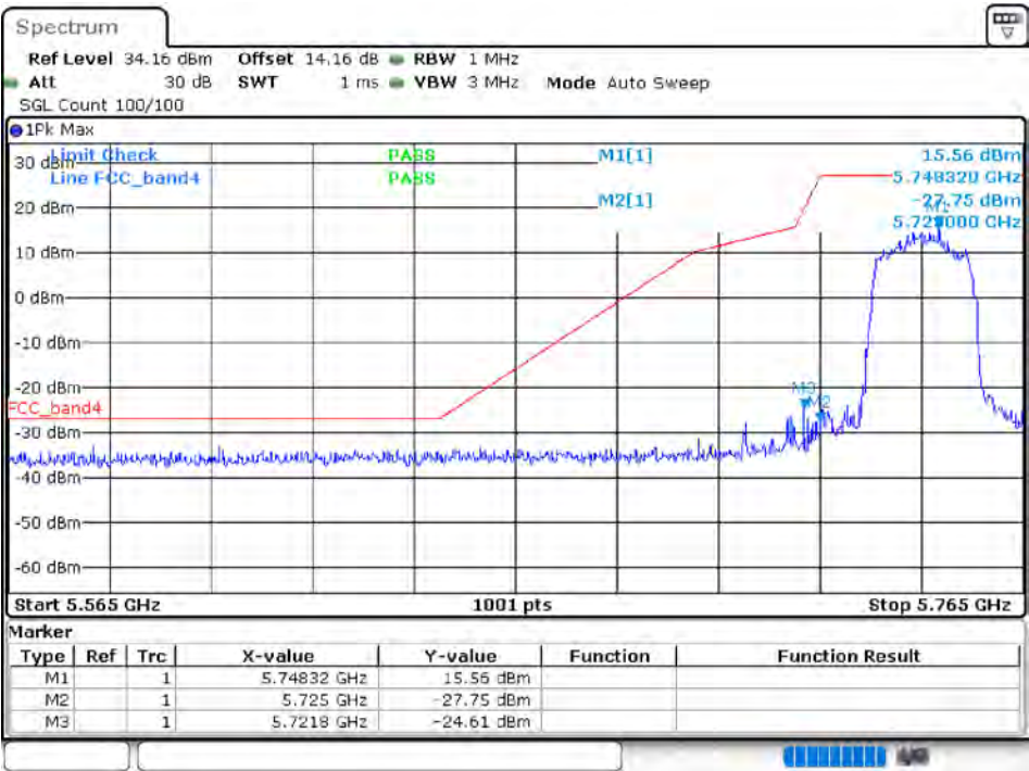
Band Edge NVNT 802.11ax20 5825MHz High Ant 1
