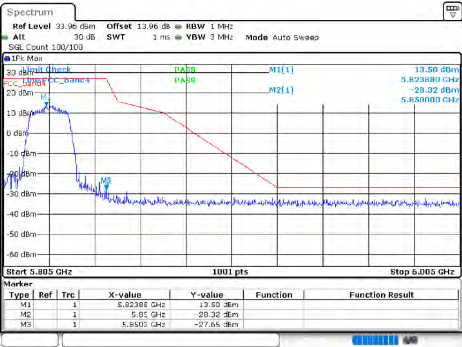
Band Edge NVNT 802.11n(HT20) 5825MHz High Ant 1
