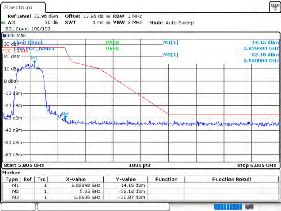
Band Edge NVNT 802.11ax20 5825MHz High Ant 1
