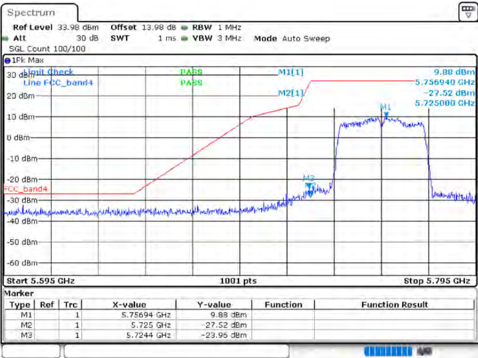
Band Edge NVNT 802.11n(HT40) 5795MHz High Ant 1
