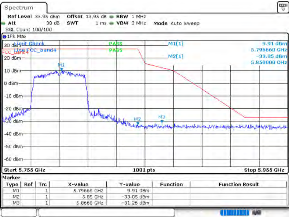
Band Edge NVNT 802.11n(HT40) 5795MHz High Ant 1
