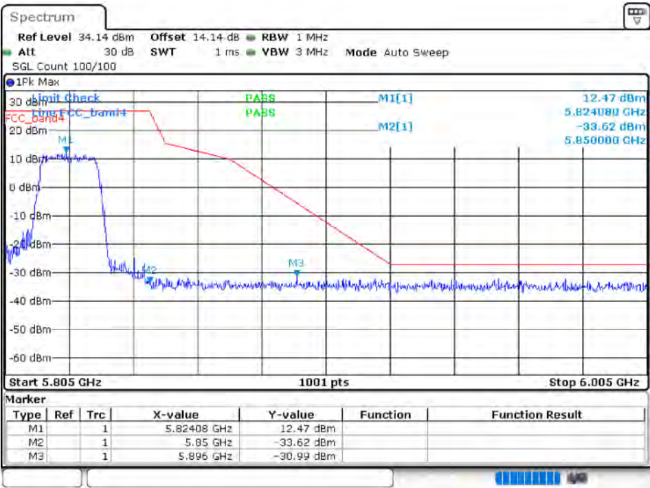
Band Edge NVNT 802.11ac20 5825MHz High Ant 2
