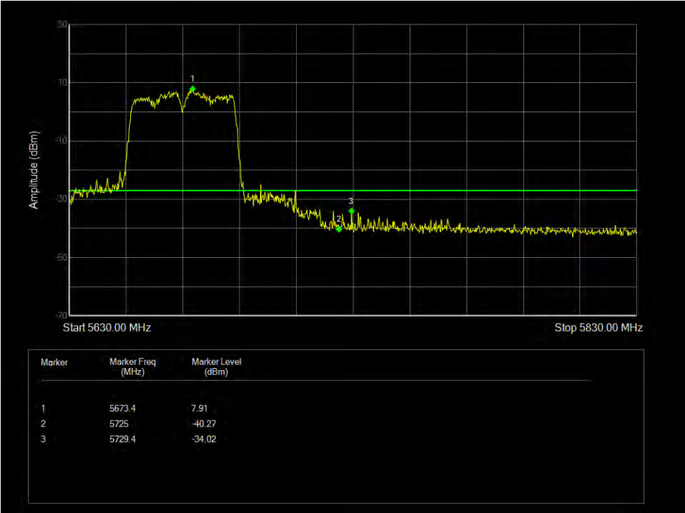
Band Edge NVNT 802.11n(HT40) 5670MHz High Sum
