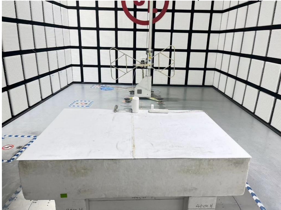
RADIATED RF MEASUREMENT SETUP (30MHz~1GHz)
