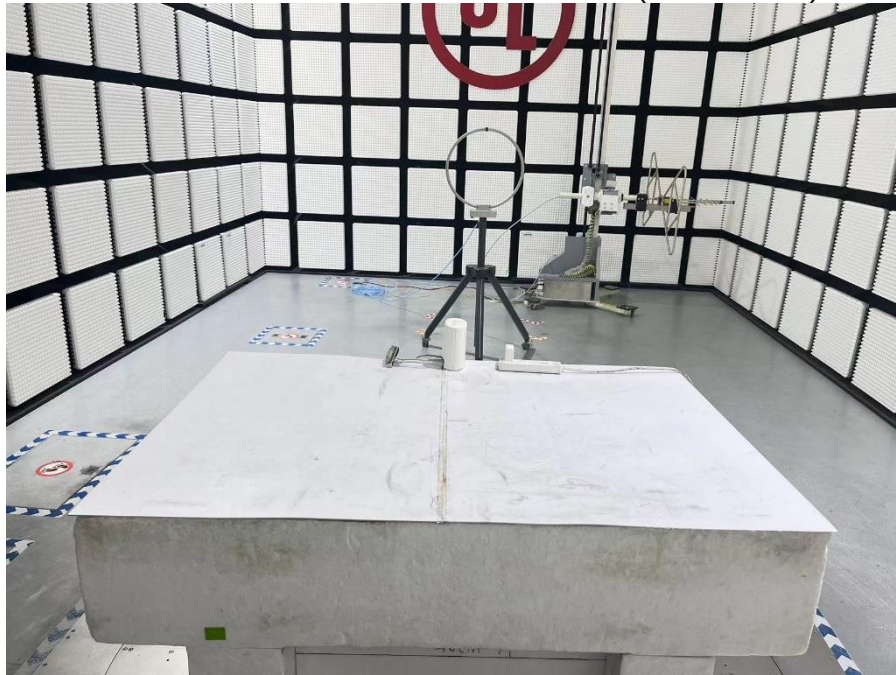
RADIATED RF MEASUREMENT SETUP (Below 1GHz)
