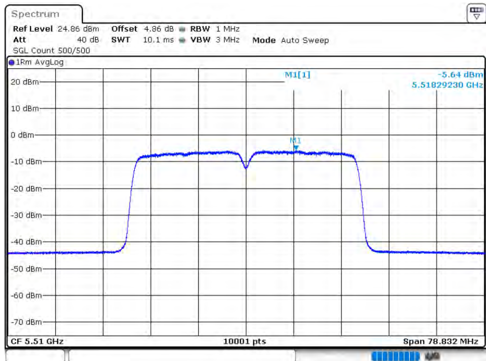
PSD NVNT 802.11n(HT40) 5510MHz Ant2
