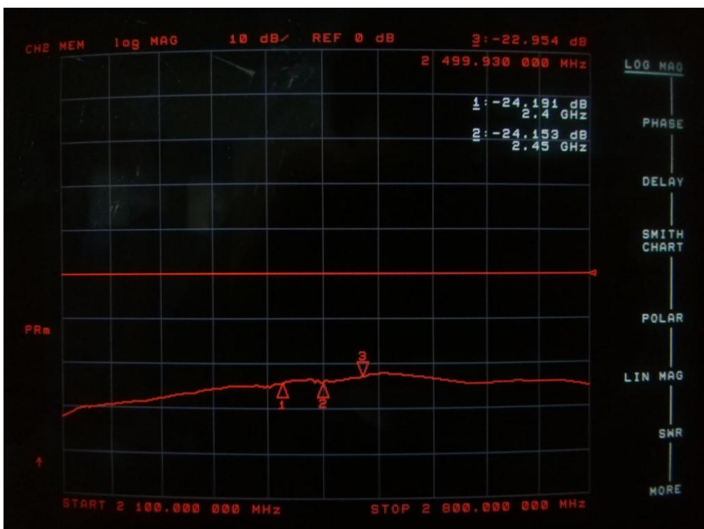
Isolation between WIFI-A and BT at 2.4G
