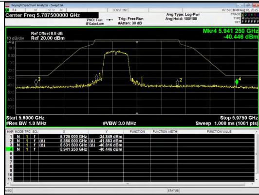
Out Of Band Emission IEEE 802.11n_Channel 151_40MHz_Antenna 0
