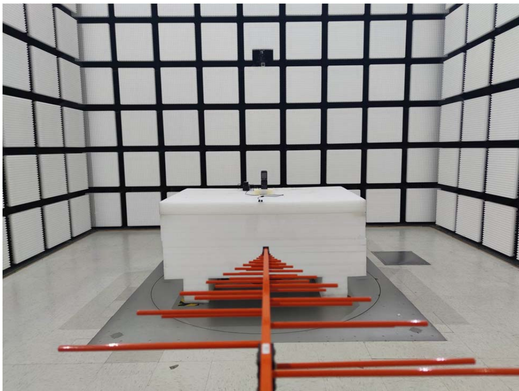
Radiated Emission 30 MHz-1 GHz View
