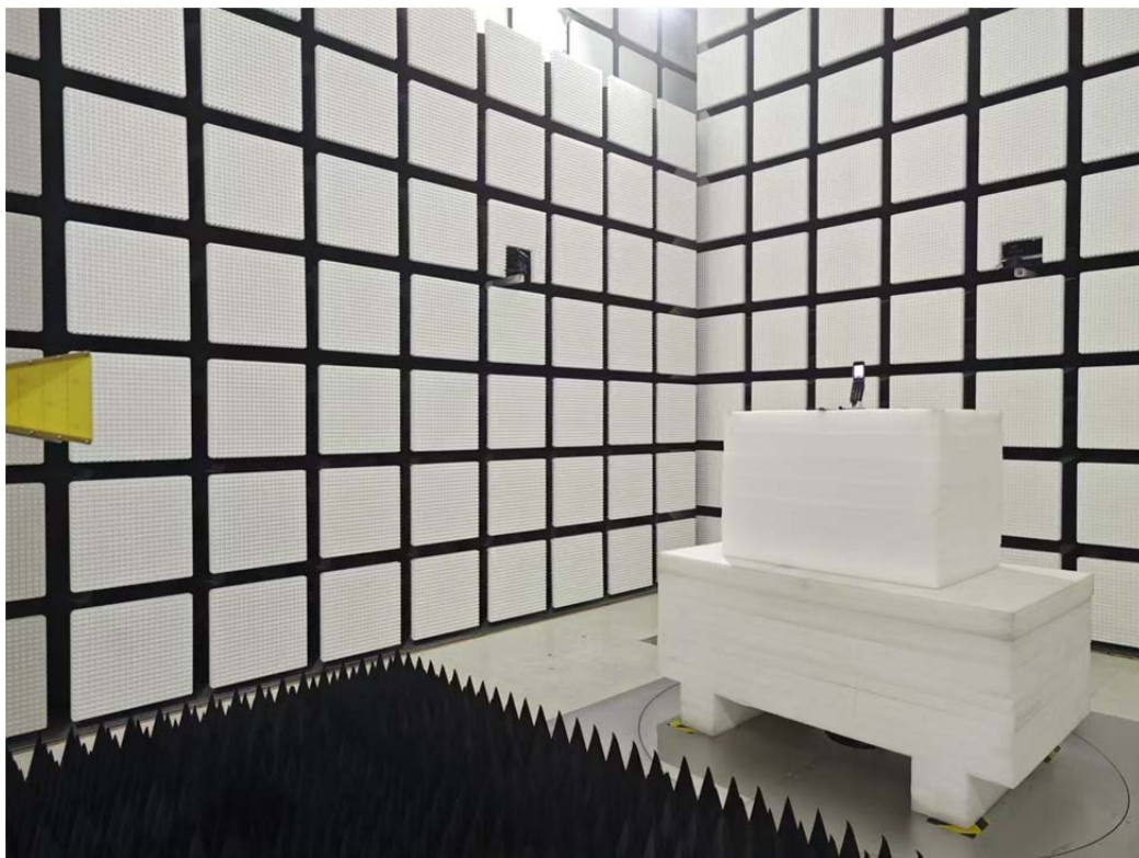
Radiated Emission Above 1GHz View 1-18G
