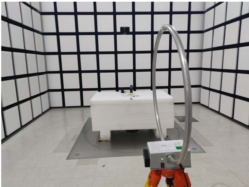
Radiated Emission 9 kHz-30 MHz Perpendicular View
