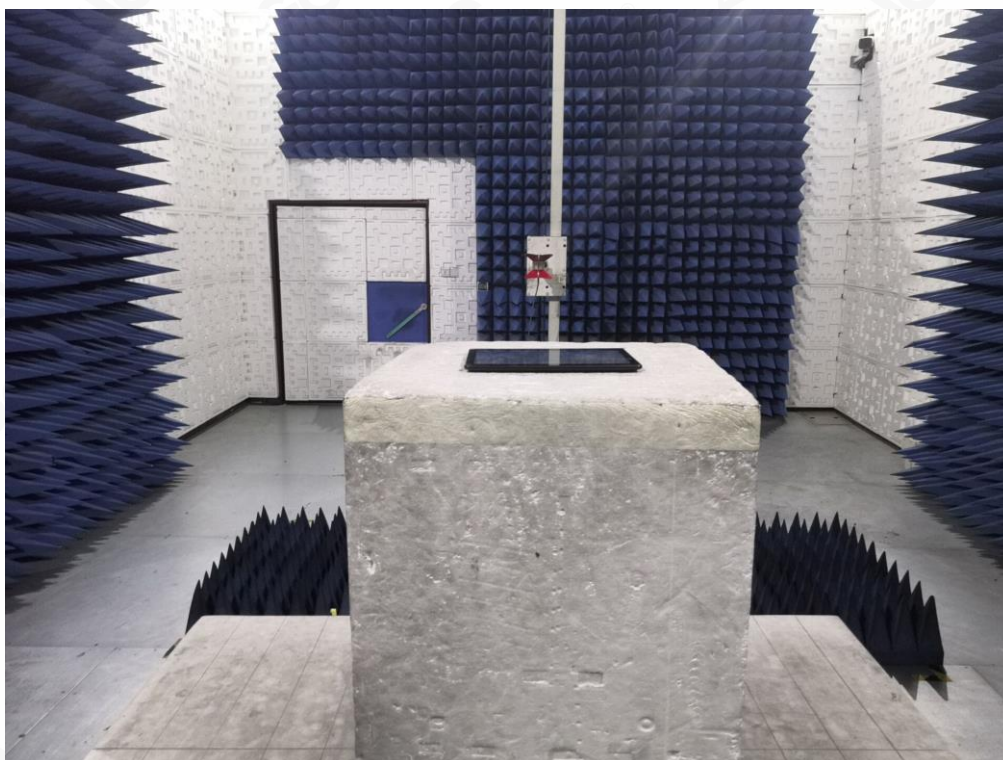
FCC RADIATED EMISSION TEST SETUP ABOVE 1GHZ
