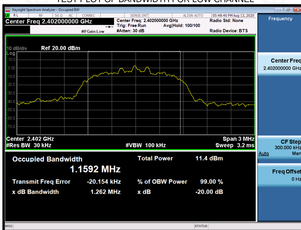
TEST PLOT OF BANDWIDTH FOR LOW CHANNEL
