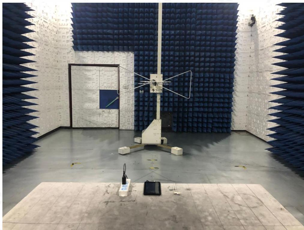
**FCC RADIATED EMISSION TEST SETUP ABOVE 1GHZ**
