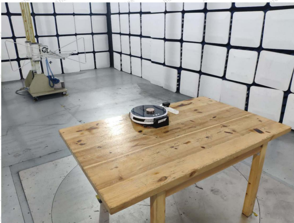
Photo of Radiation Emission Test
