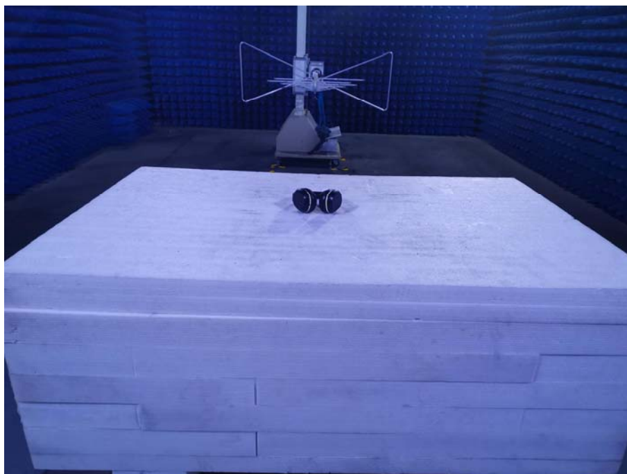
Photo of Radiated Emission Measurement (Below 1G)
