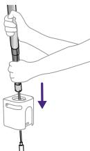
**7** Then, with the power cord first, insert the pole through **the opening of the clamp**.
