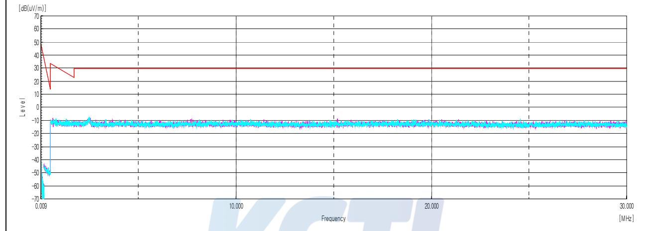
**Test results (Below 1 000 MHz) –Worst case: 1 MBits/s(37 Bytes) 2 402 MHz**
