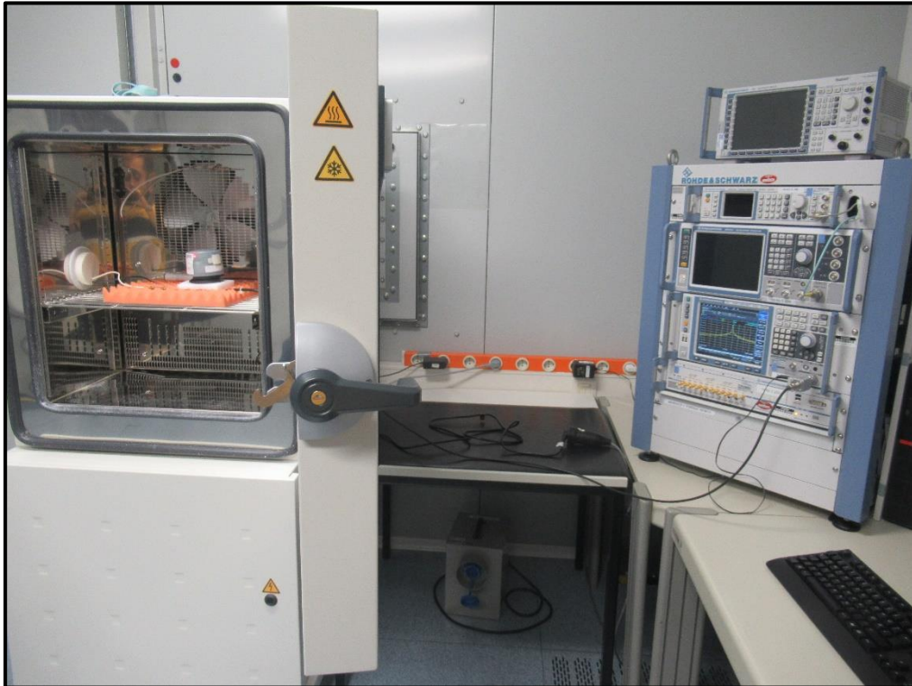
Photo 5 Bench test set up for (20 dB Bandwidth and Frequency Stability) (@ Ambient + Extreme Temperature, as required)
