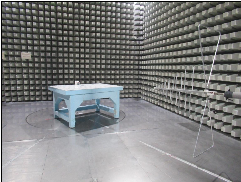
Photo 3 Radiated Test Setup from 30 MHz to 1 GHz
