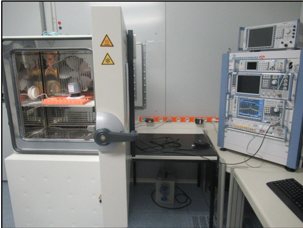
Photo 5 Bench test set up for (20 dB Bandwidth, 99% Bandwidth and Frequency Stability) (@ Ambient + Extreme Temperature, as required)
