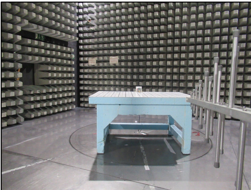
Photo 4 Radiated Test Setup from 30 MHz to 1 GHz
