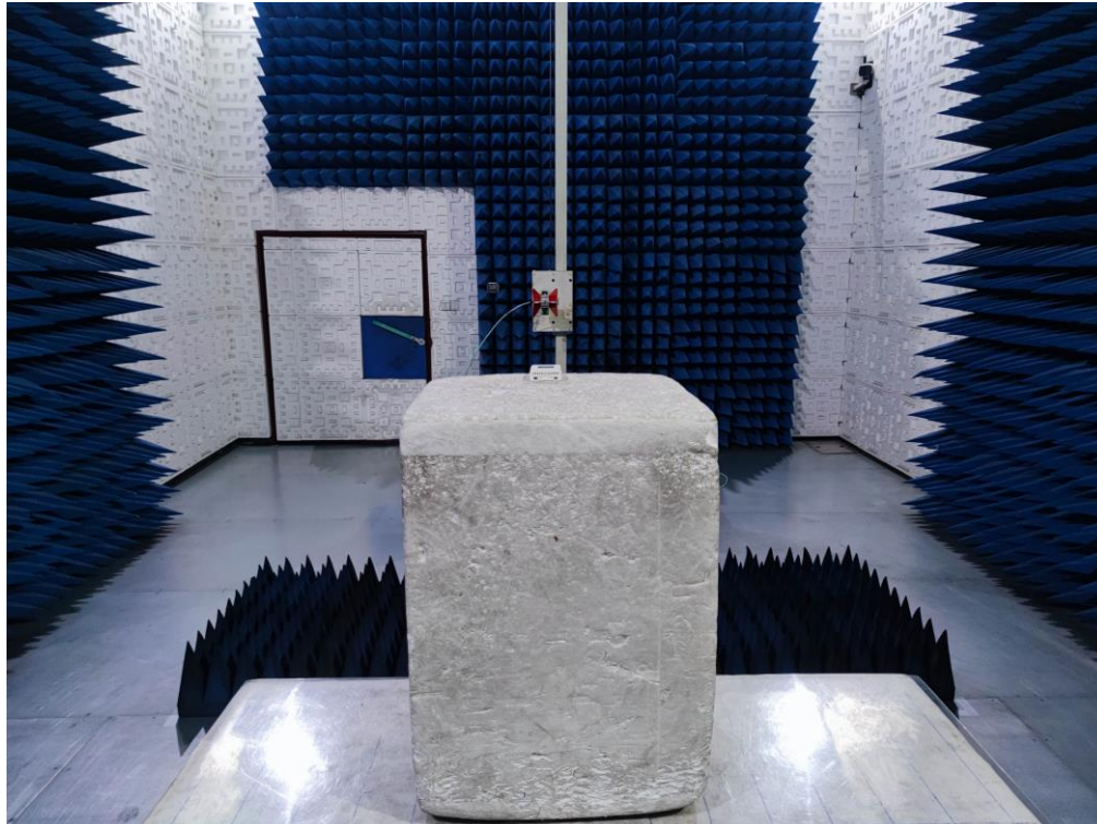
RADIATED EMISSION TEST SETUP ABOVE 1GHz
