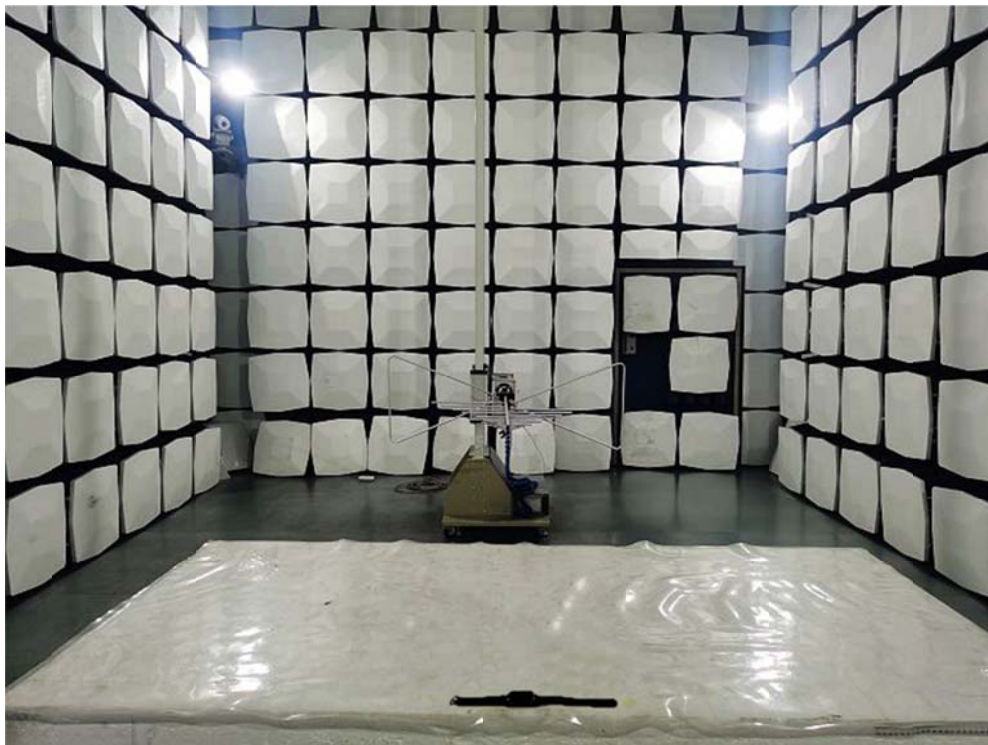
Radiated emission Test Setup
