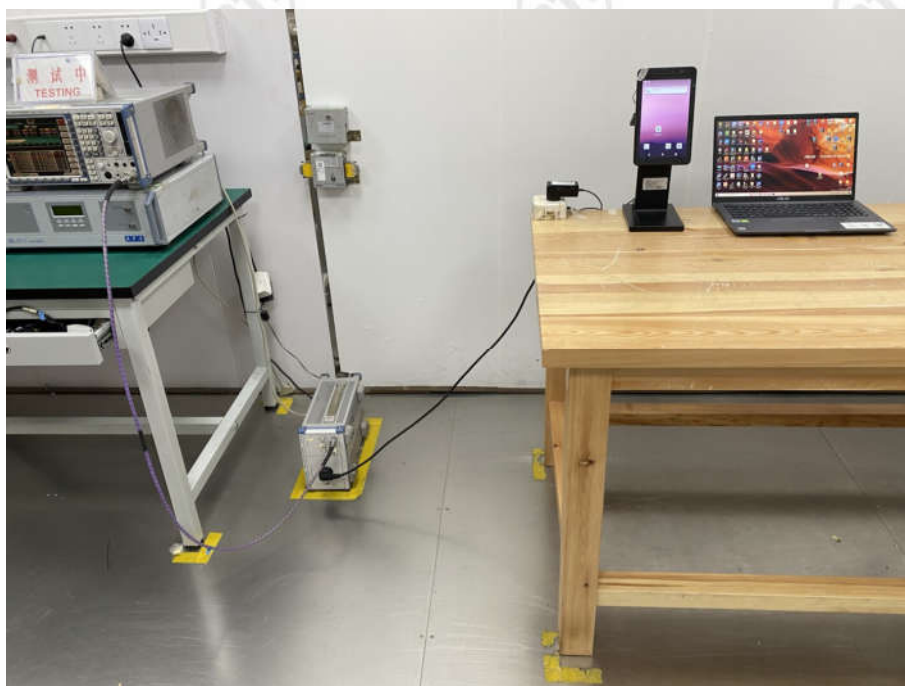
Conducted Emissions Test Setup
