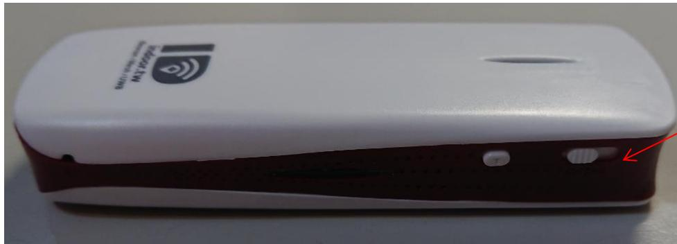
**Switch to left position to set device to be Beacon**
