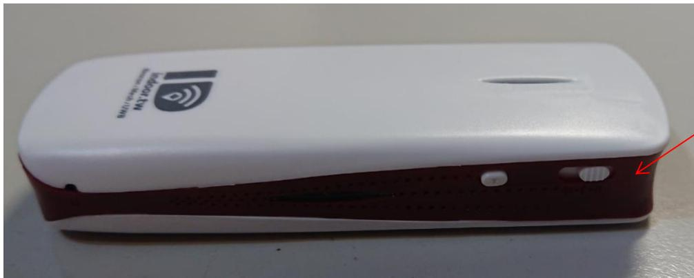
**Switch to right position to set device to be Mesh Node Relay Node 、 or Gateway Node**
