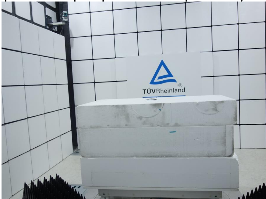
Photograph 10: Test Setup for Spurious Emissions (Front View 2)
