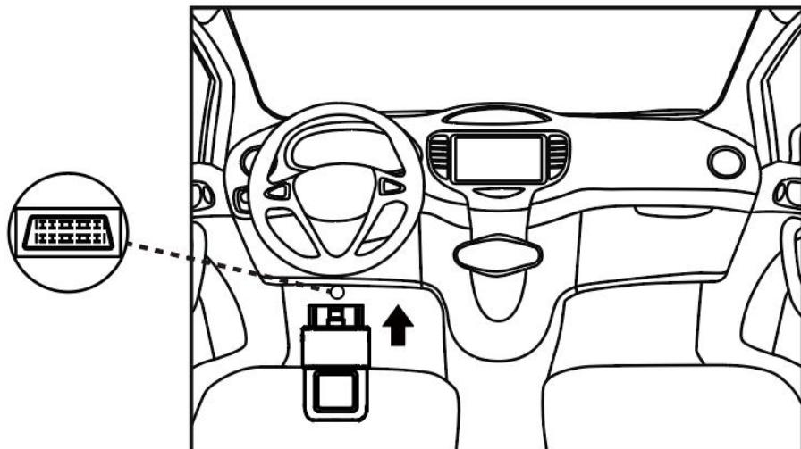
① Connect the device to the vehicle's DLC port.
