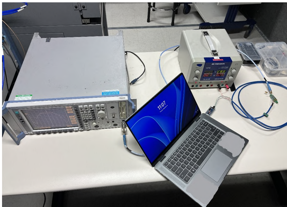
Photo 6: Test setup for conducted test, e.g. bandwidth
