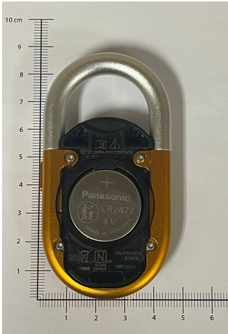
R1S keyfob back view with battery
