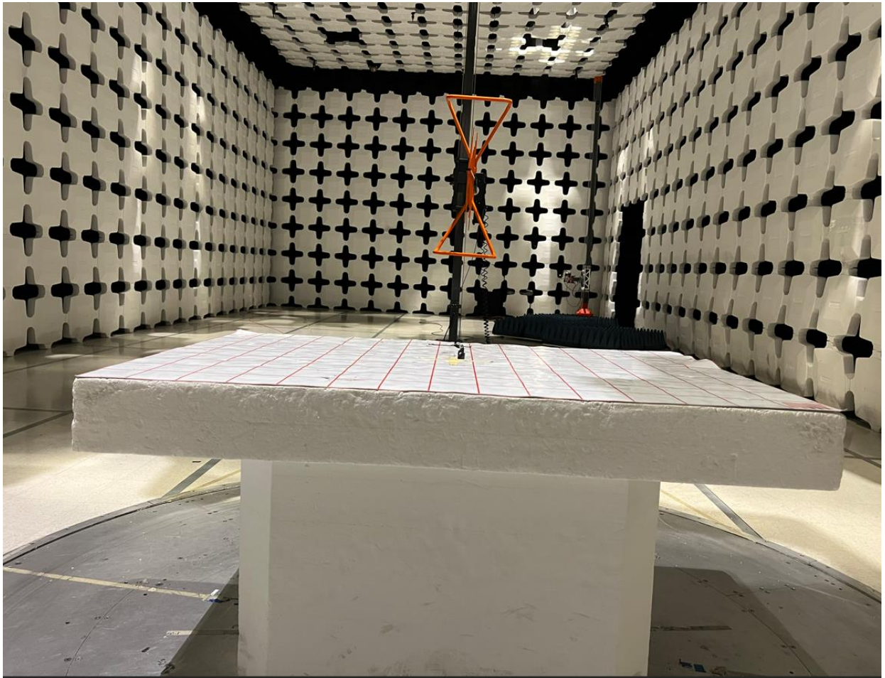
Figure 3: Test Setup for 30 MHz to 1000 MHz
