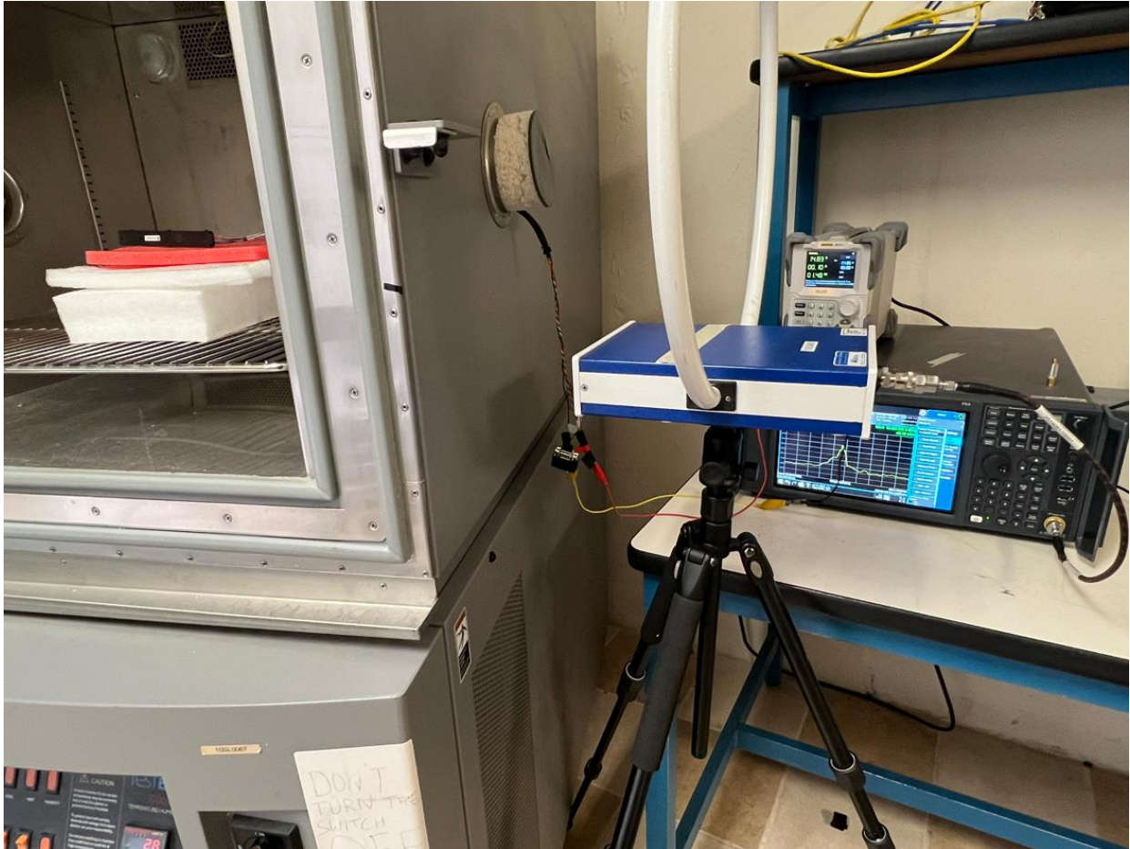
Figure 4: RF Conducted Test Setup
