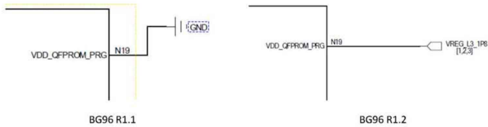
Figure 1: Schematic Designs of BG96 R1.1 and R1.2
